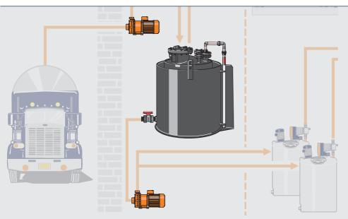
Storage tanks and dosing tanks precisely produced to customer specifications, and matching transfer pumps, guarantee safe decentralised storage and appropriate provision of process chemicals on site.
