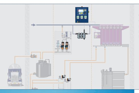
The precise interplay of metering pump, controller and sensor is a guarantee of optimum metering. Components from ProMinent are perfectly interacting and together they form a perfect control loop.
